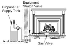
Figure 34 - Checking Gas Joints for Propane/LP Gas Fireplace
